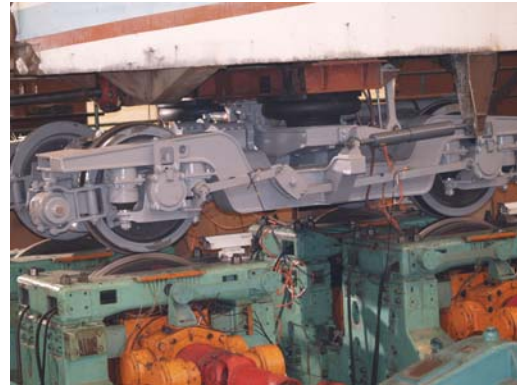
Fig. 14. Bogie system under roller rig test.
